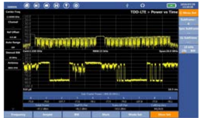
Figure 4: TDD-LTE power vs. time measurement.
