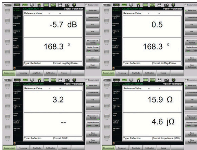
Select Which Data Display Format You Prefer, the Site Master S820E Converts the Format Automatically for You
