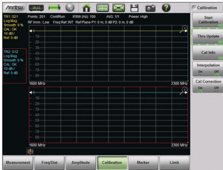
With a Simple Through Update, Measurement Errors Caused by the External Cable Drift is Removed
