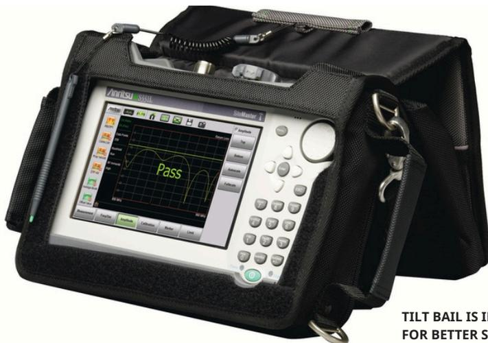
TILT BAIL IS INTEGRATED INTO THE SOFT CASE FOR BETTER SCREEN VIEWING
