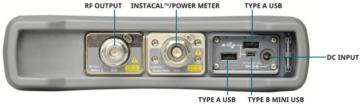
All Connectors are conveniently located on the top panel, leaving the sides clear for handheld use.
