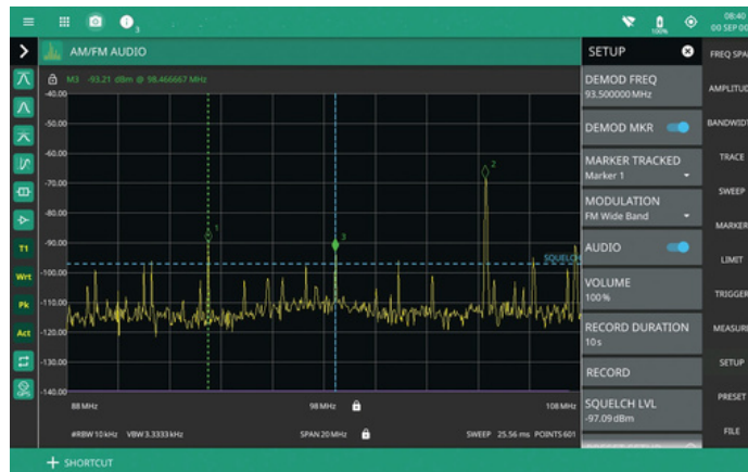
AM/FM Signal Demodulation at Marker Frequency
