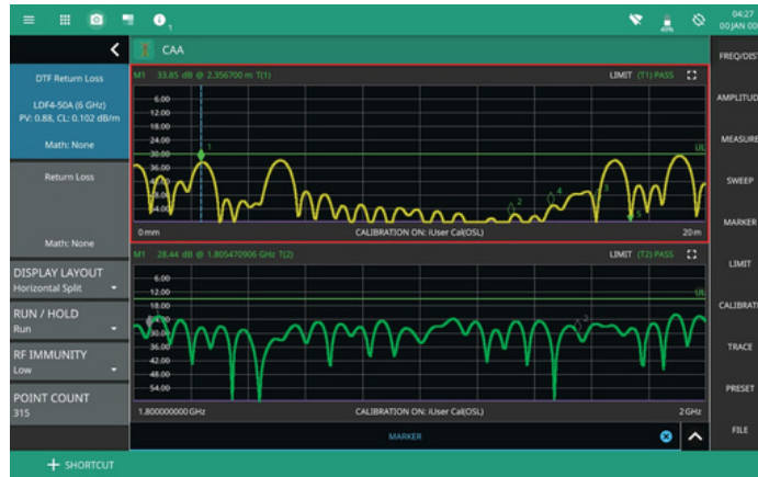
Split Screen Showing Return Loss and DTF Return Loss of a 20 Meter Cable Feed
