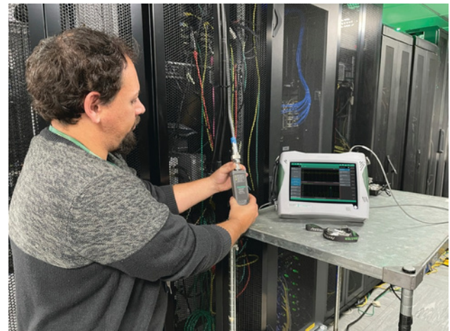
The Small Form Factor of the S331P Enables Direct Connection to the Cable Under Test Without the Need for a Test Port Cable
