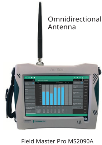
Field Master Pro MS2090A Offers Multi-PCI Measurements for OTA Testing of One or More 5G NR gNB
