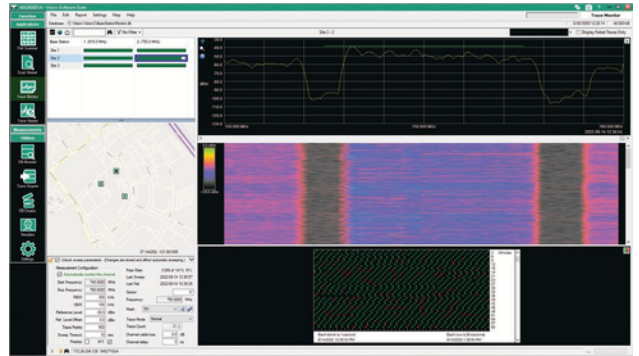
Vision Monitor Simultaneously Displays Current Spectrum, Spectrogram, and Pass/Fail History over an Extended Time Period on a Single Screen
