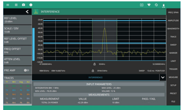
Interference Finder Option 24 Provides Fast Audio Tone Response to Changing Interference Levels
