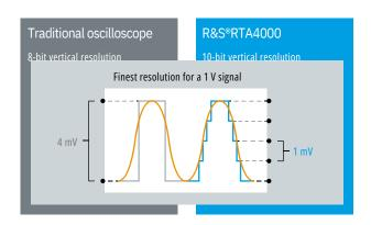
be determined during the on/off times within the same acquisition. For precise measurements of small voltage components, a high resolution of more than 8 bit is essential. With high resolution decimation, the R&S®RTA4000 even provides up to 16-bit vertical resolution, a resolution previously unseen in this class of instrument.
